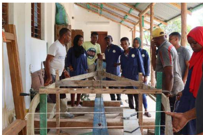
Recycled Plastic Lumber utilized for boat construction. Source: The FlipFlopi ( https://www.theflipflopi.com )
